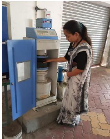
Fig 5.4: Compressive strength test
